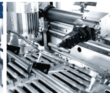
Chain feeding system with V-supports for preformed shaft parts of various shapes.
