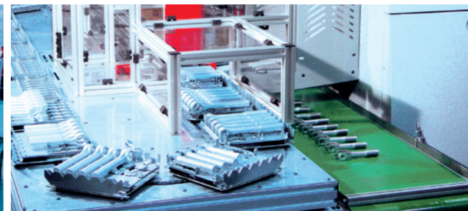
20-station pallet magazine with customer-specific pallets
